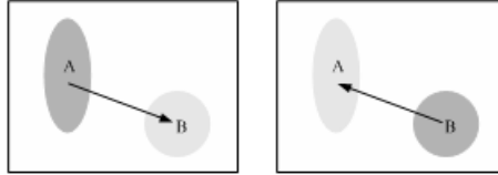
Figure 1.1 Ordinal measure of relationship between two regions. An arrow points from the darker region to the brighter one. Left: Region A is darker than B, i.e. A < B . Right: Region A is brighter than B, i.e. A > B .
