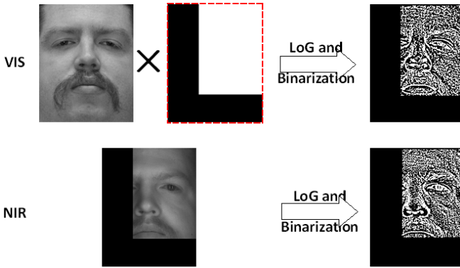
Fig. 3. NIR and VIS face images and their corresponding LoG filtered binary images
